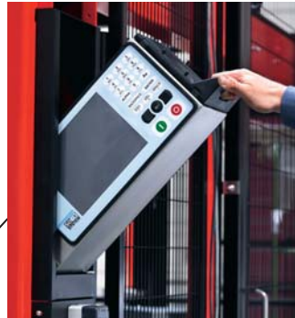
The control panel is located in one of the pillars of the robot.
